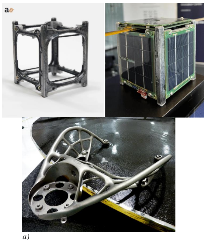
Figure 7. Additively manufactured components for aerospace industry: a) Topology optimized 3D printed composite frame for CubeSat [15]; b) 3D-printed aluminum antenna bracket for communication satellite [17].
