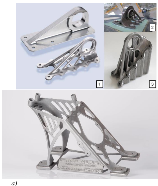
Figure 5. Additively manufactured brackets for Airbus A350 XWB:
