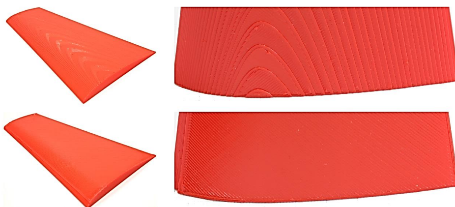
Figure 8. Comparison of a wing with NACA 4310 airfoil profile printed with planar layers (top) and a nonplanar surface (bottom) [1]
