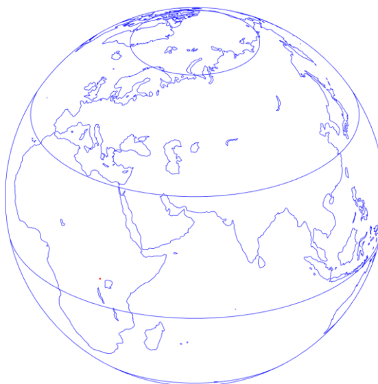
Fig. 3.7. 3D - TURKSAT 5B, Perigee argument -120^{\circ} , Right ascension of the ascending node -45^{\circ} , True anomaly -0^{\circ}
